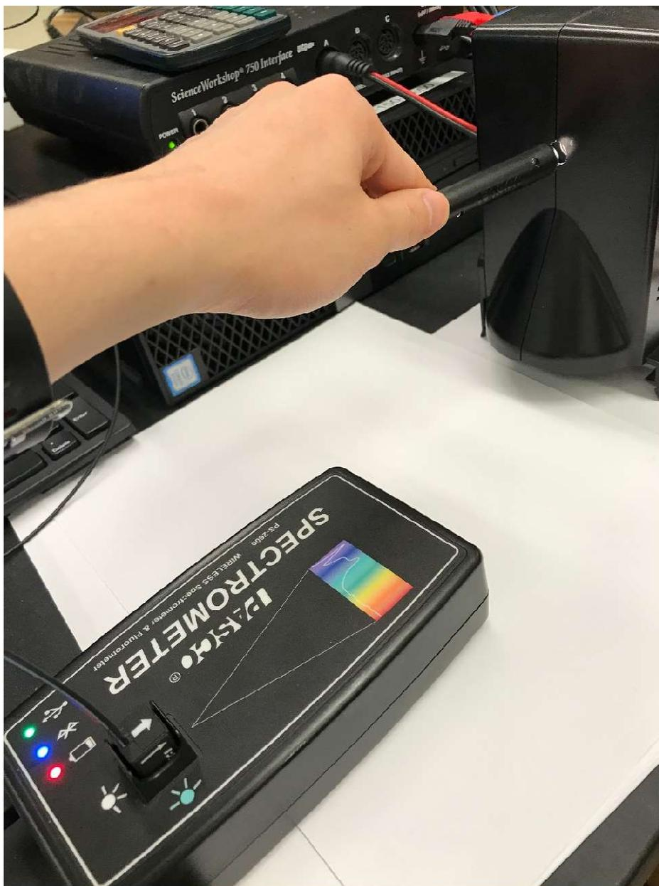
The USB Status LED should continuously shine green. (NOTE: The Bluetooth Status LED will slowly blink blue). The Battery Status LED may also blink to indicate that the battery is charging through the USB cable. We are going to use the USB connection, not the Bluetooth wireless connection between the spectrometer and the computer. The accuracy of our spectrometer (specified by the manufacturer) is approximately equal to  $\pm 2$  nm.
